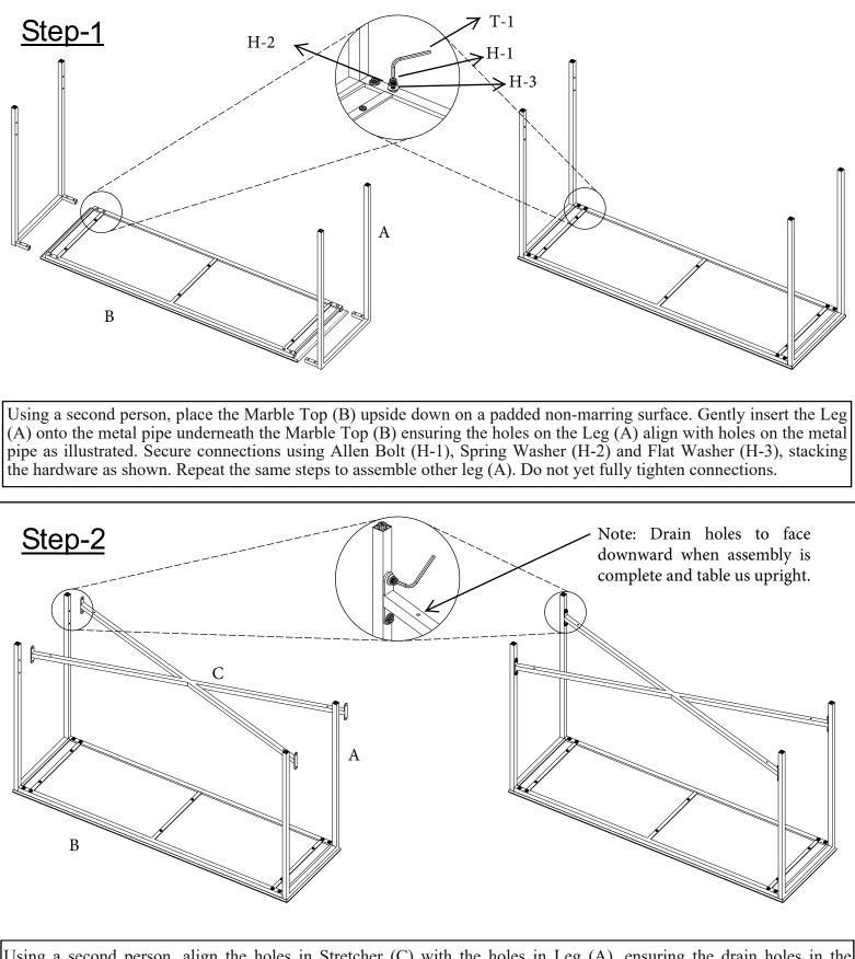
Using a second person, align the holes in Stretcher (C) with the holes in Leg (A), ensuring the drain holes in the stretcher will face downward when the assembly is complete and standing upright. Secure connections using Allen Bolts (H-1), Spring Washers (H-2) and Flat Washers (H-3). Fully tighten all connections using Allen Key (T1).
